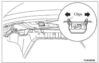
Pull both clips away from the center as shown and remove the light unit. Then remove the bulb by pulling out.
